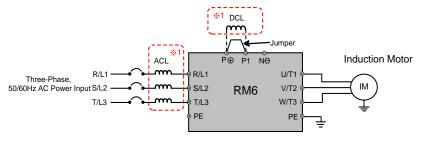
\*1,RM6-100HP above drives: AC reactor (ACL) is the standard accessory; RM6-175HP above drives: DC reactor (DCL) is the standard accessory.
